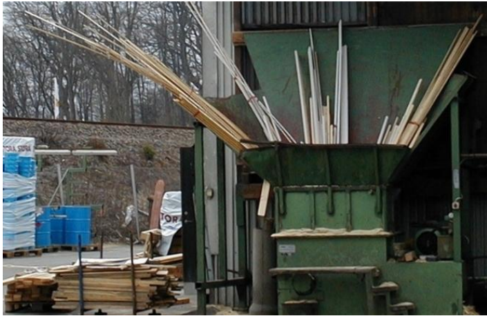
Compacting waste – the most valuable wood products are fillets – by milling to chips because of quality reasons.
